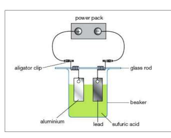
**9** Carefully pour enough 1.5 mol/L sulphuric acid into the beaker to almost cover both pieces of metal. Leave about 1 cm above the surface.
