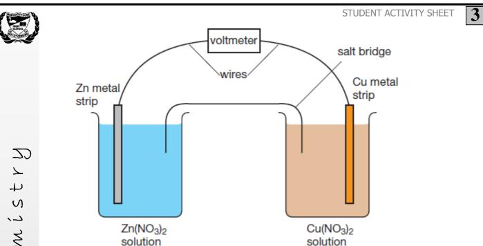
**5** Use the connecting wires to connect the zinc metal and copper metal to the voltmeter as shown in the diagram above. You may need to swap the wires on the voltmeter to get a reading. Note which electrode (metal) is positive and the magnitude of the voltage; record these observations in the results table.
